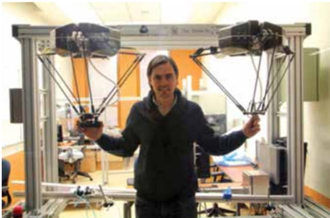
Juan Pablo Martínez from Automatische Technik, the first Mexican company to create industrial delta robots, its robotic applications are mainly focused on packing, unpacking and repacking any type of products into boxes.
